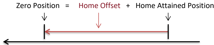
Figure 8-35: Setting Zero Position Utilizing Home Offset
